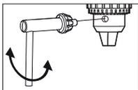
**NOTE:** Never use a wrench or means other than a chuck key to tighten or loosen the chuck.
