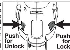
To **unlock** the trigger, push the trigger lock as shown.
