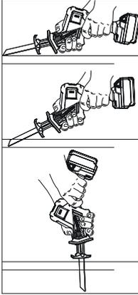
1. Insert the blade into the tool with the teeth facing down. Hold the tool as shown, resting the edge of the shoe on the workpiece.
