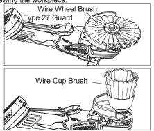
Test wheel for balance and loose or damaged wires by letting it spin for one minute before applying it to the workpiece. During this time, no one should stand in front of or in line with it.
