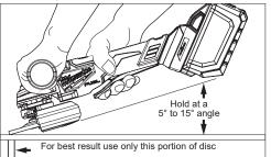
**Cross Sanding** - When finishing a surface that has been prepared by a coarse disc or wheel, sand at right angles to the strokes made by the coarser disc. Finishing marks left from previous sanding are easily seen and removed for a uniform finish. Failure to cross sand when changing from a coarse disc to a finishing disc may result in deep scratches and circular marks.
