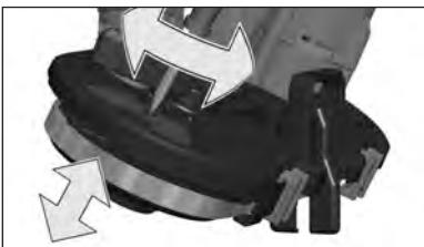
If necessary, adjust blade tracking.
