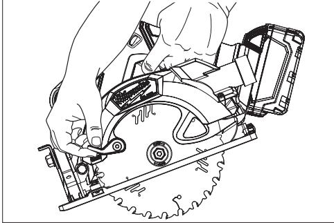
2. To start the saw, push the lock-off button down while pulling the trigger. Allow the motor to reach full speed before beginning cut. Using the front of the shoe as a hinge point, gradually lower the back end of the saw into the workpiece. Release the lower guard lever and grasp the front handle.
