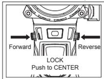
3. To **lock** the trigger, push the control switch to the center position. The trigger will not work while the control switch is in the center locked position. Always remove the battery pack before performing maintenance or changing accessories. Always lock the trigger or remove the battery pack before storing the tool and any time the tool is not in use.
