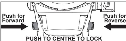
1. For **forward** (clockwise) rotation, push the control switch in the direction shown. Check the direction of rotation before use.
