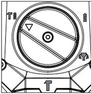
**NOTE:** To engage the hammering mechanism, maintain pressure on the bit. When pressure on the bit is released, the hammering action will stop.
