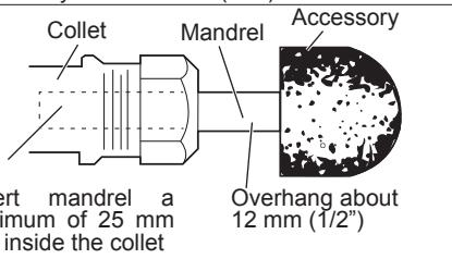
4. Press in the spindle lock button while turning the collet nut clockwise. Tighten securely.
