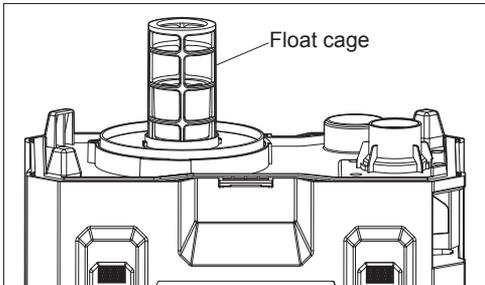
3. A float cage shuts off suction when the tank is full. Be sure that the float is clean and moves freely in the float cage to ensure that the float valve works.
