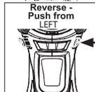
To **lock** the trigger, push the control switch to the center position. The trigger will not work while the control switch is in the center locked position. Always lock the trigger or remove the battery pack before performing maintenance, changing accessories, storing the tool and any time the tool is not in use.
