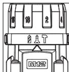
Then rotate the torque selector collar until the desired clutch setting appears in line with the arrow.
