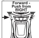
For **reverse** (counterclockwise) rotation, push in the control switch from the left side of the tool. **Check direction of rotation before use.**
